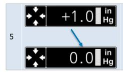
**Zero the Pressure Displays** This sets the pressure gauges to local conditions. See page 48.
