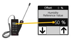
Change the Reference Value to match the Reference Device reading.
