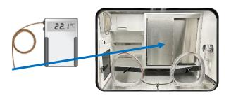
Insert the sensor for the reference device that measures temperature into incubator and allow incubator temperature reading to settle for at least one hour after the reading has stabilized.
