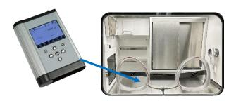
Insert the sensor for the reference device that measures oxygen into workspace and allow workspace oxygen reading to settle for at least one hour after the reading has stabilized.
