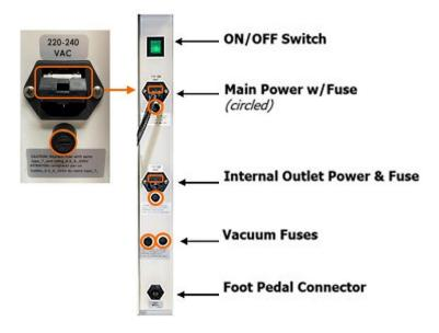
**Note**: The BACTRON400HP is delivered with all fuses installed. Replace fuses with the same type of fuse. Insert the correct power cords.
