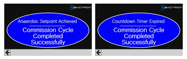
**Note**: The oxygen setpoint that the Anaerobic Commissioning stops at is 400 ppm. This is not adjustable by the operator. However, the Anaerobic Alarm indicator is an adjustable setting.
