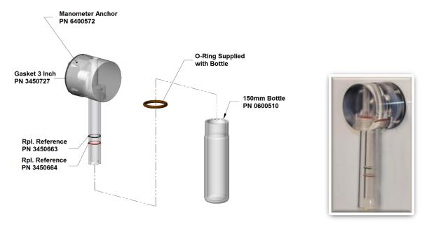
Figure 9: Chamber Manometer
