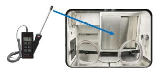
Insert the sensor for the reference device that measures relative humidity into incubator and allow incubator relative humidity reading to settle for at least one hour after the reading has stabilized.
