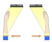
This position prevents the collapsing sleeves from pulling your hands into the arm port doors during the vacuum down cycle phases. It also keeps the sleeve material tight, helping to obtain a complete evacuation of the sleeves.
