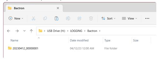
Find the newest folder. At this point you can copy the folder from the SD Card to your hard drive or open the folder and copy individual csv files to your hard drive. Each comma separated log file will contain up to 24 hours of data. If the datalogger is stopped and started or the Bactron is turned off then on, the datalogger starts a new comma separated log file.
